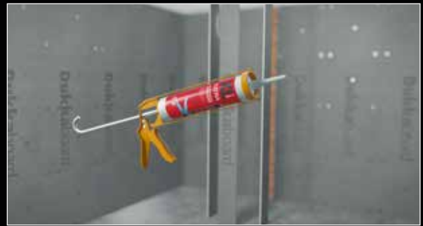
4. On adjoining edges run a continuous bead of Dukkaboard XL glue. Applying glue to one surface only is sufficient.
